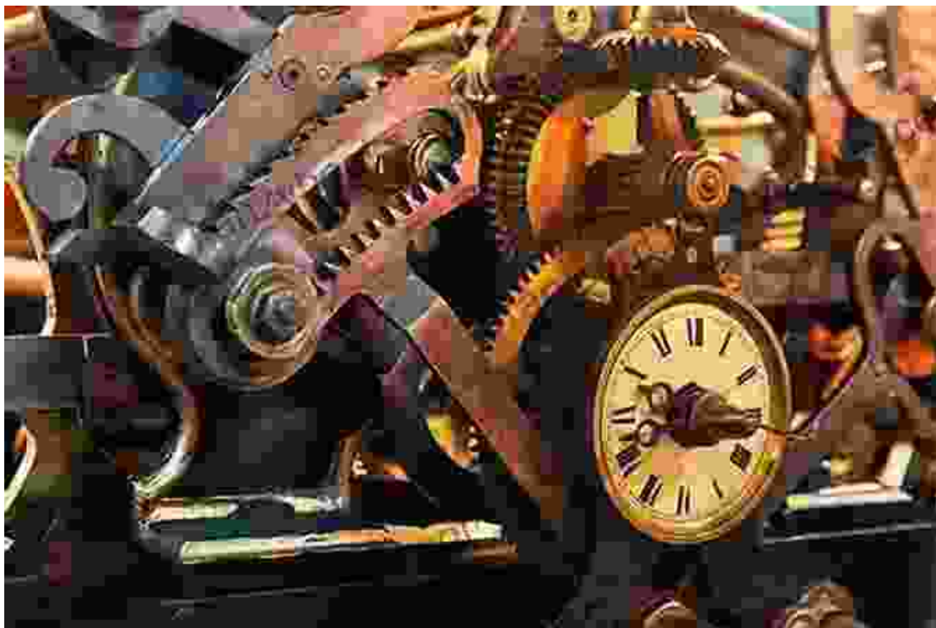
Mechanical clock using a weight to power a gear train
